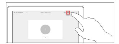
8. Tap the **camera icon** in using the soft key on the upper right of the Touch 10 pad to adjust the in-room camera view. The Self-view is the default camera position. Adjust the camera position with the tilt, pan, and zoom controls.
