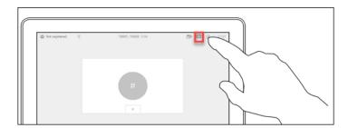
13. Tap the **camera icon** in using the soft key on the upper right of the Touch 10 pad to adjust the in-room camera view. The Selfview is the default camera position. Adjust the camera position with the tilt, pan, and zoom controls.
