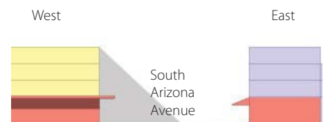
Buildings located on the west side of South Arizona Avenue to block hot afternoon summer sun.
