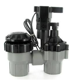
Your system may be using a different type of backflow preventer, they are called anti-siphon valves. Each valve has a type of backflow preventer built in. While these are compliant with codes, they cannot be tested so they are not the preferred method. Over time the gravity operated seal can become stuck in the closed position giving a false sense of protection. These valves are also installed above ground and need to be protected from the sun and any other accidental damage.
